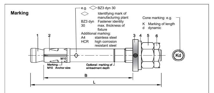
Usable length:  $B = h_{ef} + t_{fix}$
